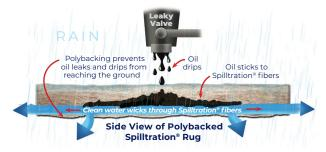
Spilltration® Husky Polyback Products have two sides. A thick, absorbent Spilltration® fiber top side captures oil and allows clean water to filter through; and a leak-proof polymer backing prevents oil leaks from reaching the ground.
